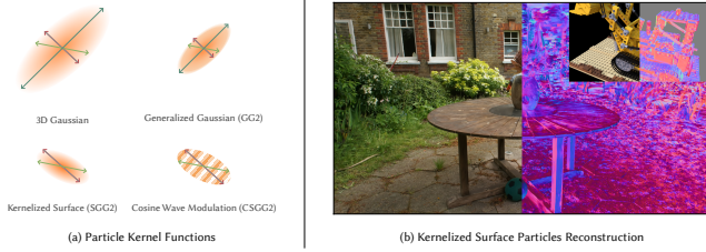
Fig. 6. Particle Kernel Functions: (a) In addition to 3D Gaussians, in this work we investigated three other particle types: the generalized Gaussian (GG2), kernelized surface (SGG2) and cosine wave modulation (CSGG2) particles. (b) Shows radiance and normal reconstructions obtained with the kernelized surface particles for two scenes.
