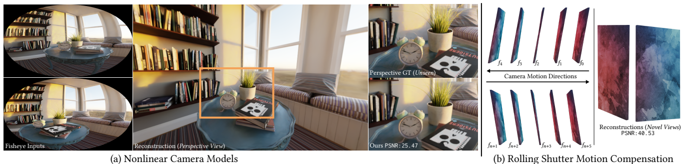
Fig. 15. Complex Cameras: (a) Compared to rasterization-based approaches, our ray tracing-based formulation naturally supports complex camera models as inputs like distorted fisheye lenses (left), which can be re-rendered using different camera models like regular perspective cameras (right), achieving high reconstruction quality relative to unseen references (see insets (•) - this synthetic cozyroom scene is by [Ma et al. 2021]). (b) Ray tracing also naturally enables compensating for time-dependent effects like rolling shutter imagine sensors, which induce distortions due to sensor motion. This effect is illustrated on the left by multiple different frame tiles f_i of a single solid box rendered by a left- and right-panning rolling shutter camera with a top-to-bottom shutter direction. By incorporating time-dependent per-pixel poses in the reconstruction, our method faithfully recuperates the true undistorted geometry (right).
