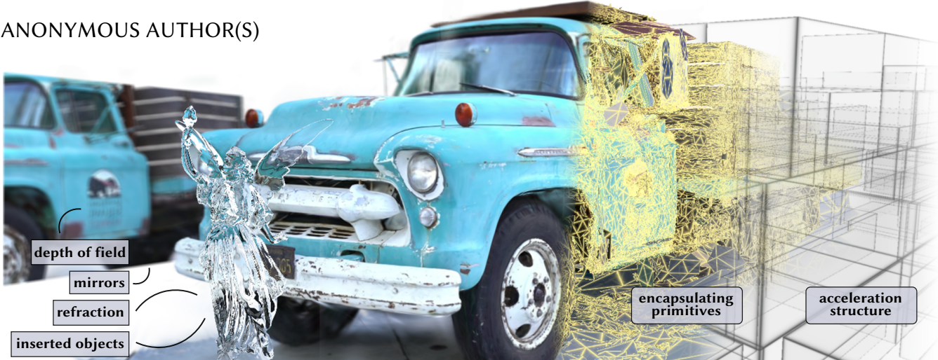
Fig. 1. We propose a method for fast forward and inverse ray tracing of particle-based scene representations such as Gaussians. The main idea is to construct encapsulating primitives around each particle, and insert them into a BVH to be rendered by a ray tracer specially adapted to the high density of overlapping particles. Efficient ray tracing opens the door to many advanced techniques in computer graphics and vision, including secondary ray effects like mirrors, refractions and shadows, as well as highly-distorted cameras with rolling shutter effects and even stochastic sampling of rays.
