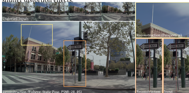
Fig. 16. AV Scene Reconstruction: Real-world AV and robotics applications often have to respect both distorted intrinsic camera models and are, at the same time, affected by time-dependent effects like rolling shutter distortions as frames are exposed at high sensor speeds. Our ray tracing-based reconstruction is well-suited to handle both challenges simultaneously, which we illustrated by an example of a side-facing top-to-bottom rolling shutter camera on an AV vehicle: the top inset (•) depicts faithful removal of the intrinsic camera model distortion by rendering with an undistorted camera, while the bottom inset (•) shows our ability to remove the apparent rolling-shutter distortions of the inputs by rendering from a static camera pose (linear indicators (•) exemplify the complex distortion of the inputs).
