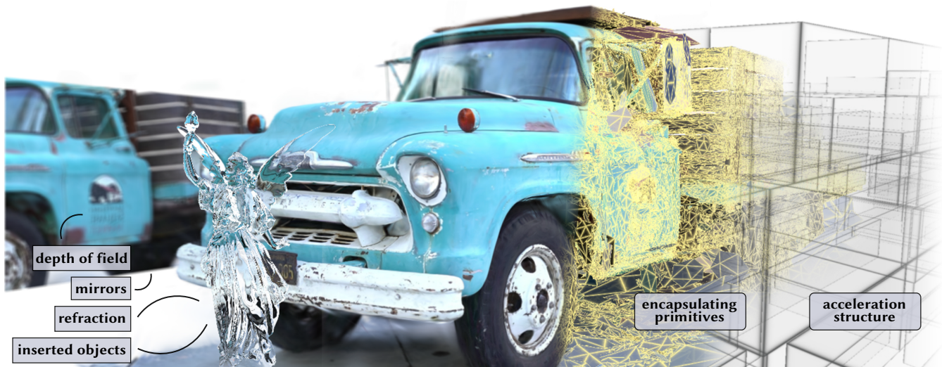
Fig. 1. We propose a method for fast forward and inverse ray tracing of particle-based scene representations such as Gaussians. The main idea is to construct encapsulating primitives around each particle, and insert them into a BVH to be rendered by a ray tracer specially adapted to the high density of overlapping particles. Efficient ray tracing opens the door to many advanced techniques, including secondary ray effects like mirrors, refractions and shadows, as well as highly-distorted cameras with rolling shutter effects and even stochastic sampling of rays. Project page: GaussianTracer.github.io
