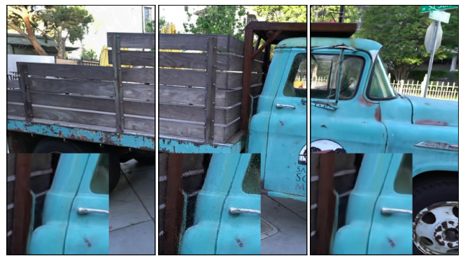
Fig. 15. Stochastic Sampling: Left, scene rendered with our proposed algorithm. Center, rendered with stochastic sampling (4 samples). Right, denoised with the NVIDIA OptiX denoiser.
