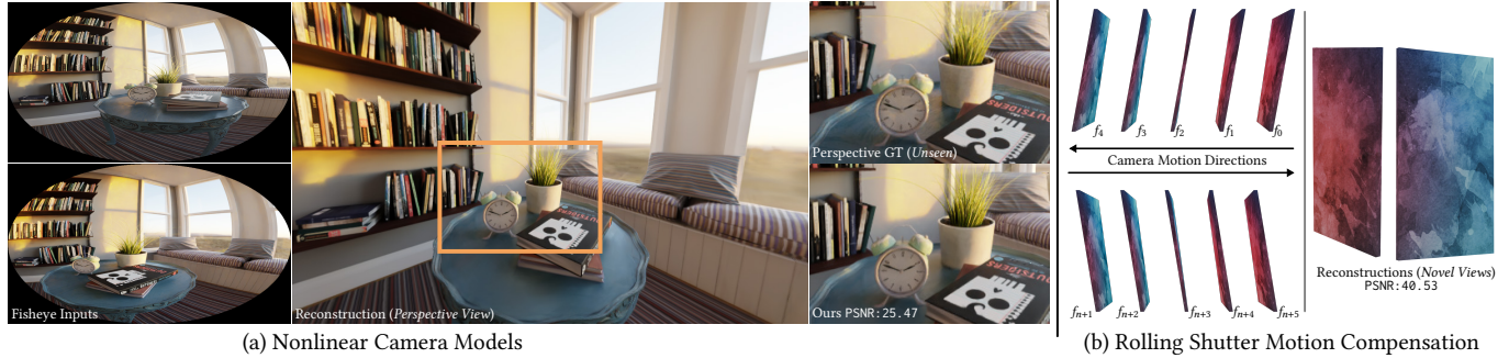
Fig. 16. Complex Cameras: (a) Compared to rasterization-based approaches, our ray tracing-based formulation naturally supports complex camera models as inputs like distorted fisheye lenses (left), which can be re-rendered using different camera models like regular perspective cameras (right), achieving high reconstruction quality relative to unseen references (see insets (•) - this synthetic cozyroom scene is by [Ma et al. 2021]). (b) Ray tracing also naturally enables compensating for time-dependent effects like rolling shutter image sensors, which induce distortions due to sensor motion. This effect is illustrated on the left by multiple different frame tiles f_i of a single solid box rendered by a left- and right-panning rolling shutter camera with a top-to-bottom shutter direction. By incorporating time-dependent per-pixel poses in the reconstruction, our method faithfully recuperates the true undistorted geometry (right).
